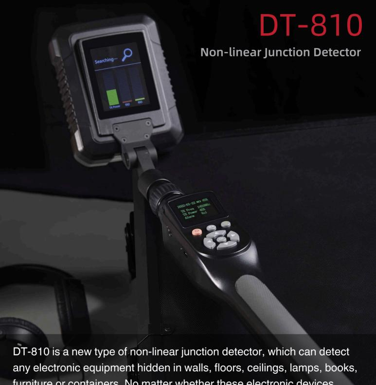
DT-810 is a new type of non-linear junction detector, which can detect any electronic equipment hidden in walls, floors, ceilings, lamps, books, furniture or containers. No matter whether these electronic devices are transmitting signals or starting up, they can alarm through display, vibration and sound prompt, so that the detector can focus on the hidden target.
