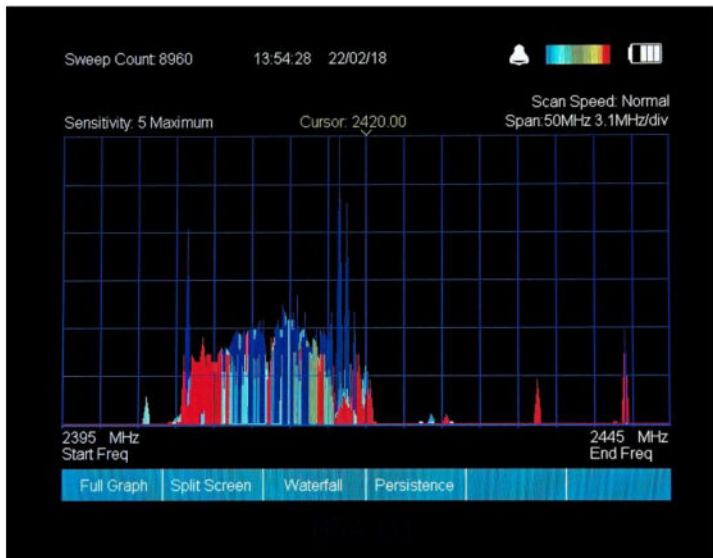
Persistence Mode – Blue signals are the least persistent, running through to Red for the most persistent.
